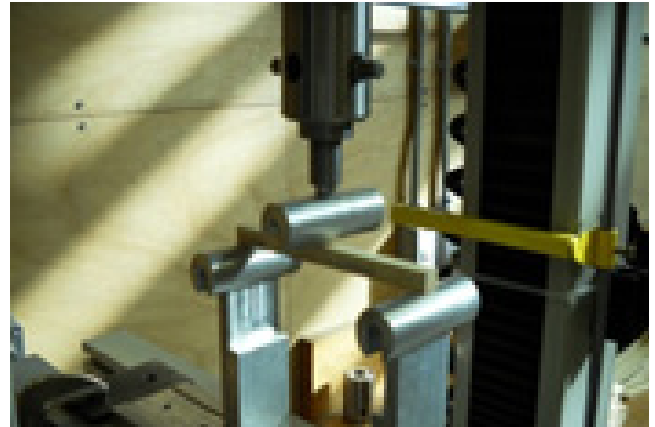
Figure 1. Bending tests to determine wood stiffness. A key wood quality trait being examined as part of the PhD study.
